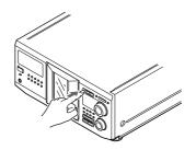
**3** Turn the JOG dial until you find the disc slot where you want to insert a disc, while checking the disc number (written beside every slot and also indicated in the small display).
